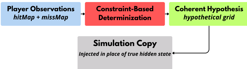
Figure 3.2: The constraint-based determinization pipeline. Accumulated hits and misses are used as spatial constraints to guide hypothesis generation. The engine produces a coherent hypothetical opponent grid that is injected into the simulation copy instead of the true hidden state.
